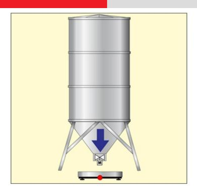
Configuration which allows to manage a dosage system in loading of a single product, useful for filling hoppers, silos or big bags, or guiding the operator in the manual dosages.
