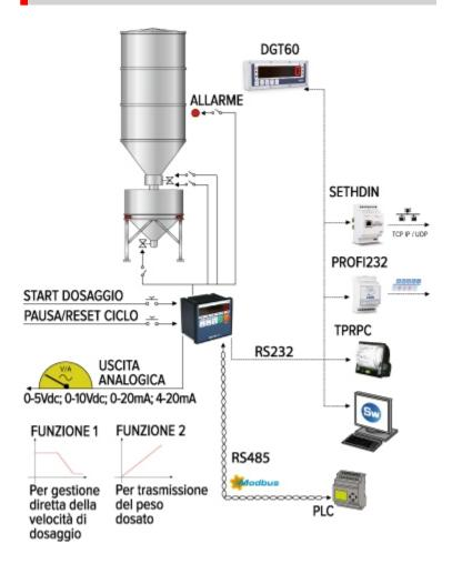
Example of dosage system usign the DGTQF for loading routine
