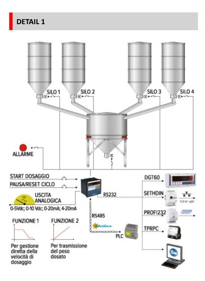
Example of dosage system using the DGTQF for loading routine
